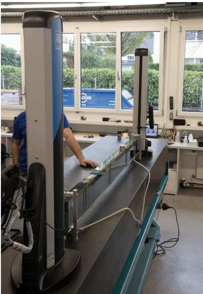
The TESA MICRO-HITEs are used on both sides of the guide and they measure different characteristics.
