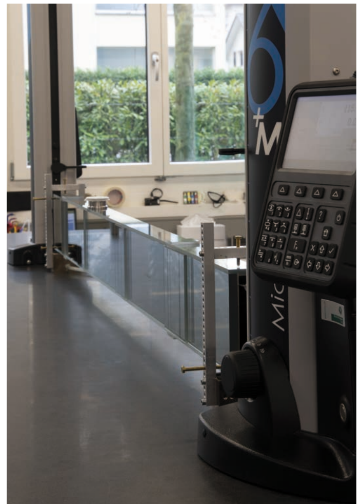
The TESA MICRO-HITEs are used on both sides of the guide and they measure different characteristics.
