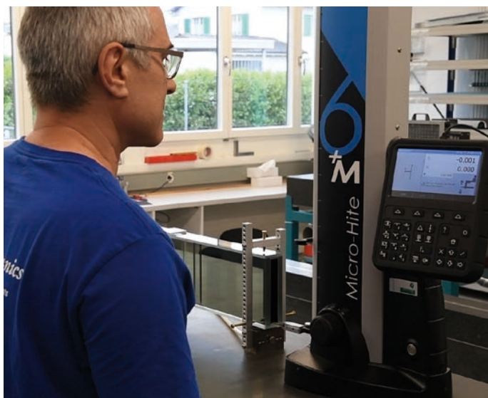
Mr. Brisacher realizing a perpendicularity measurement.
