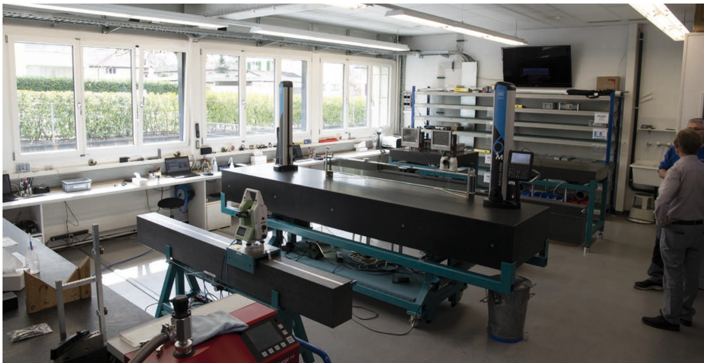
In the assembly cell for the guides two motorised TESA MICRO-HITE are used in order to ensure that the subgroups are well matched together.
