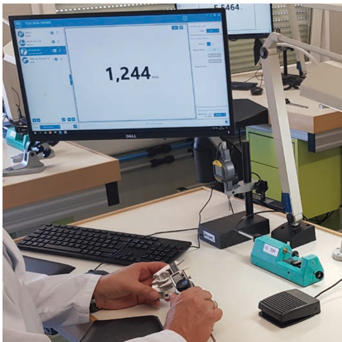
Instruments with wireless connection to the TESA DATA-VIEWER software
