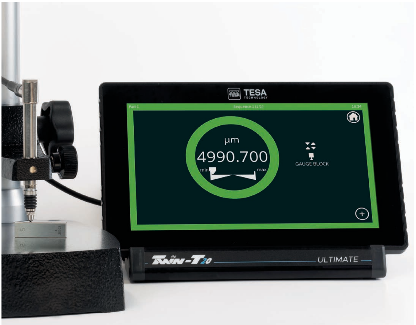
Measuring a gauge block on polished marble with a display of 0.001 μm from the connected inductive probe
