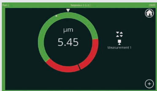
Rotating indicator display, one value
