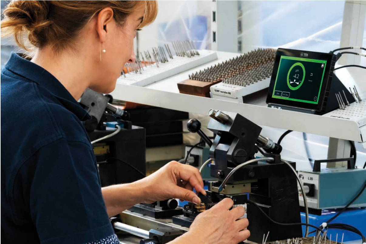
Concentricity measurement before assembly of cylindrical parts
