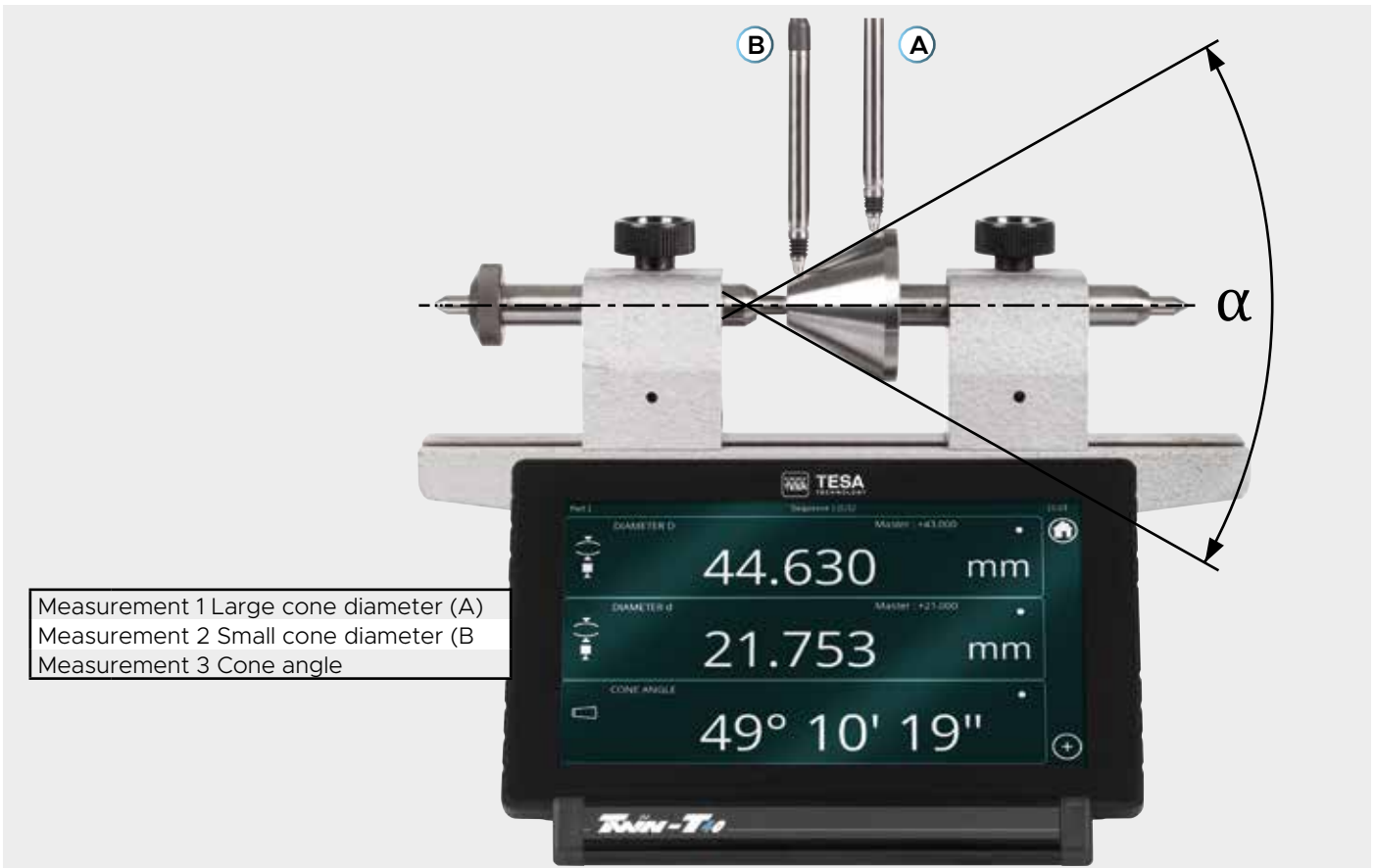
Measurement of cone angle using trigonometric functions.
