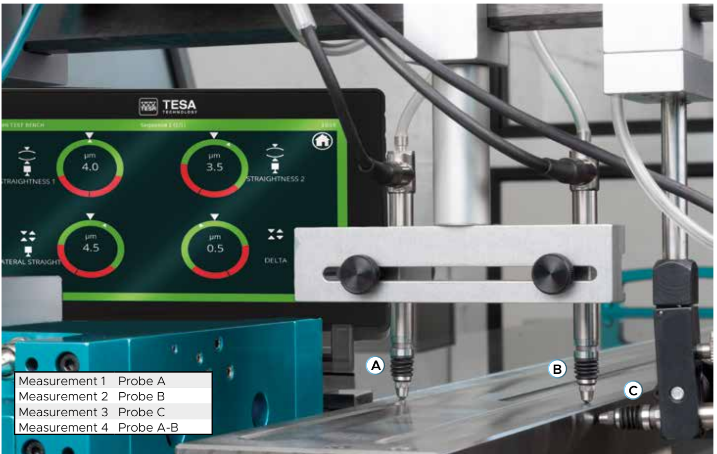
Flatness measurement in two axes simultaneously.
