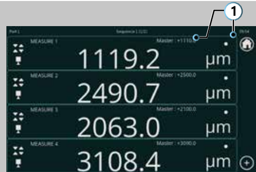
"Digital indicator" display type, four measurements
