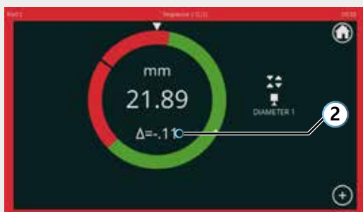
"Rotating indicator" display type, one measurement
