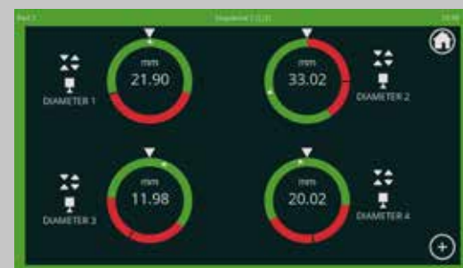
"Rotating indicators" display type, four measurements
