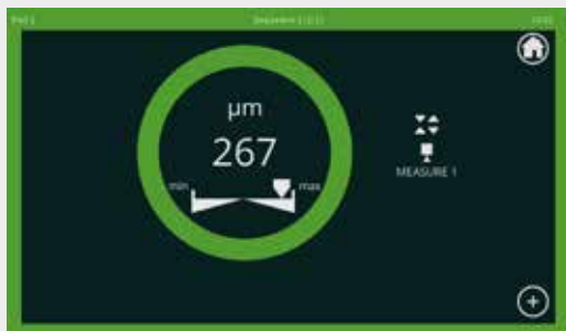
"Circular indicators" display type, one measurement
