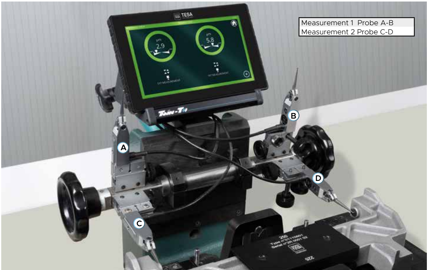
Parallelism check with GT31 electronic lever probes.
