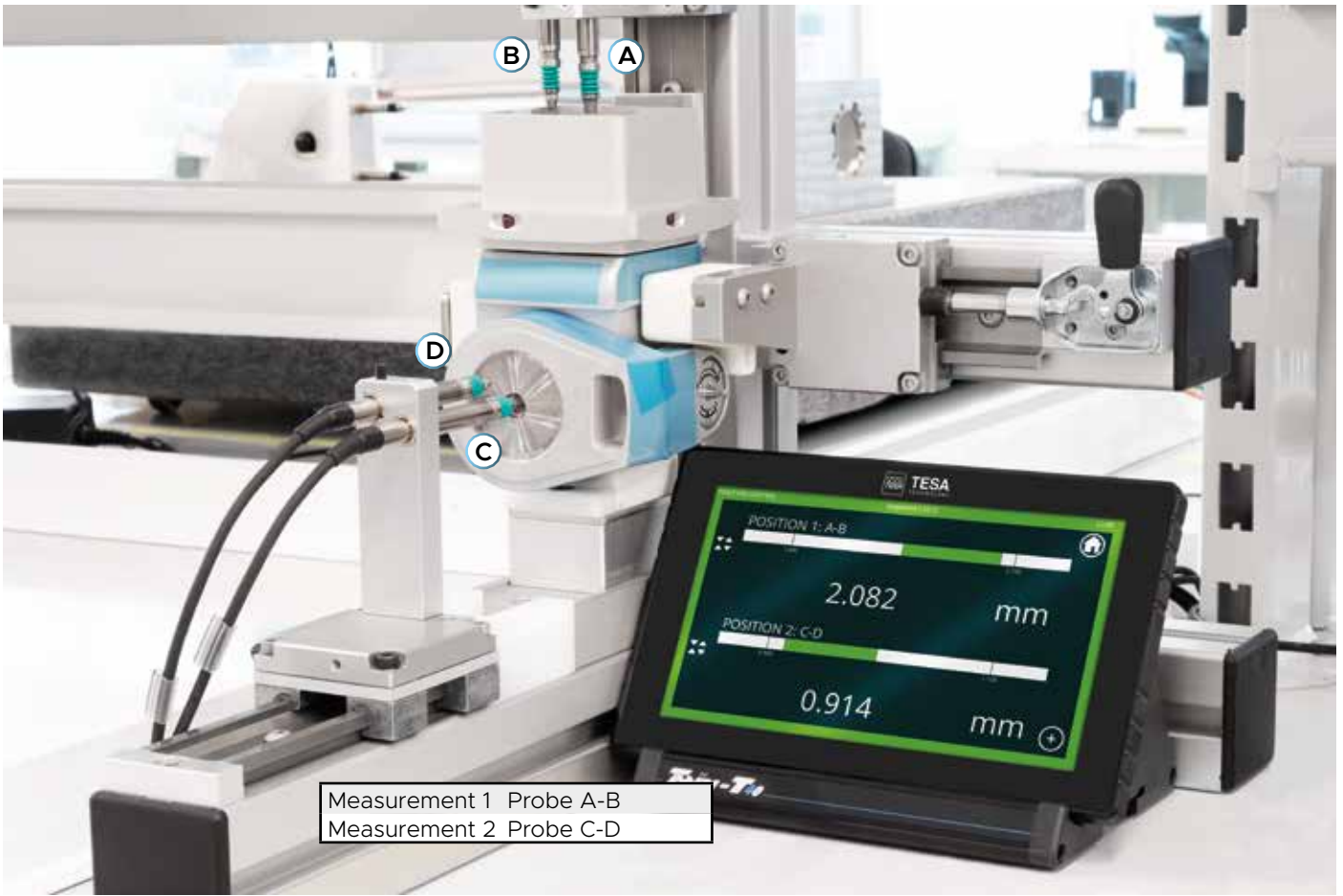
Position control during an assembly operation.
