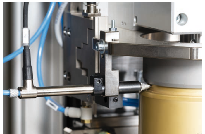
Measurement using a probe with pneumatic actuation
