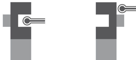
Calibration with groove of the master piece
