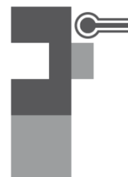
Calibration with rib of the master piece
